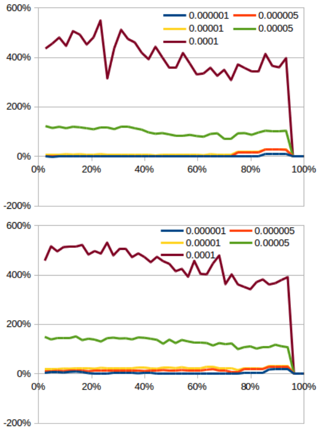
Fig. 4: Outer matvec and preconditioner application faults with decreasing l^2 -norm for the ARMS preconditioner (top) and ILUT preconditioner (bottom). On y - and x -axis, % of extra iterations and of fault-commencing iteration, respectively, compared to the number of iterations in the fault-free run.
